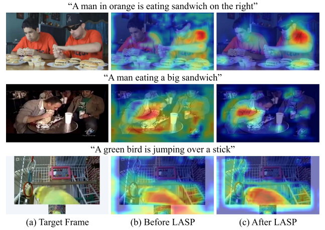
Fig. 6. Visualization of feature maps in LASP. (a) Target frames. (b) Feature activations before LASP modules. (c) Feature activations after LASP modules.
