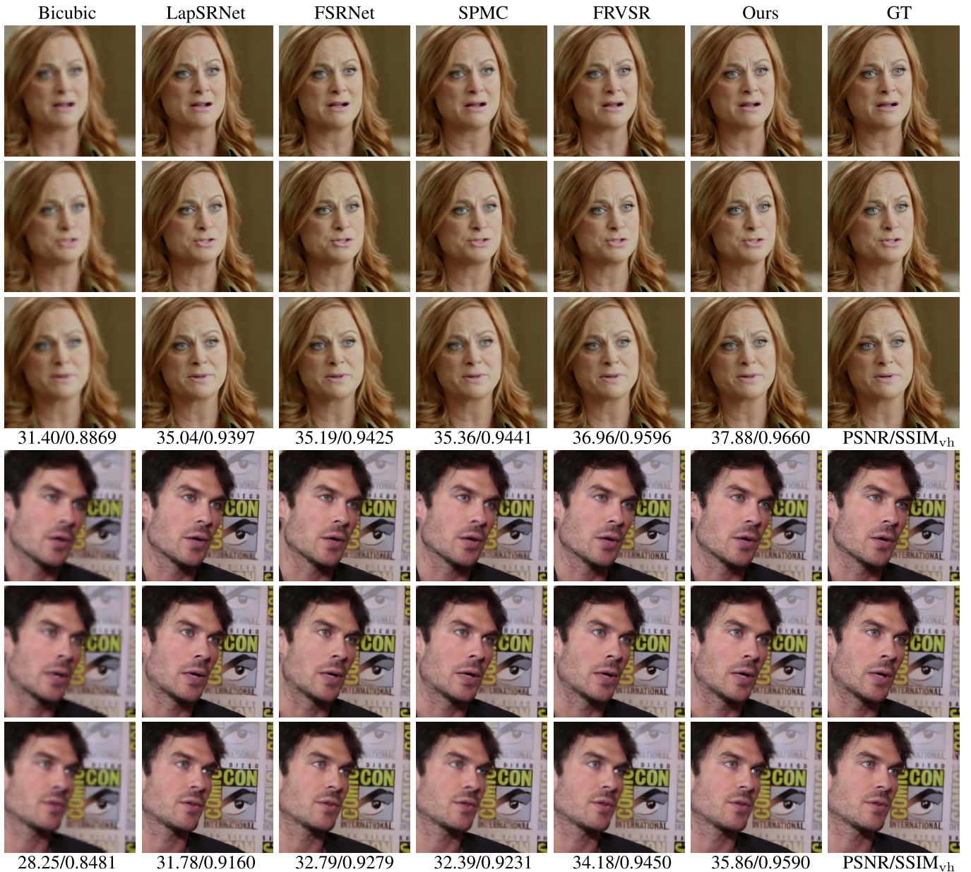
Fig. 6. Comparison of super-resolution algorithms in two facial image sequences. The predicted SR images from our method ('Ours') are closer to the ground truth than other algorithms.
