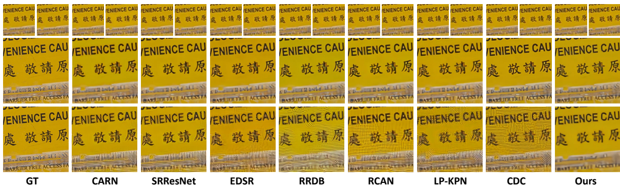
Figure 5: Super-resolved results of our proposed method and existing SR methods on the RealSR dataset. The leftmost column shows the ground truth. For other columns, the left of the first row is a clean image, while the right image is the adversarial sample with the intensity \alpha = 8/255 . The middle row is the super-resolved output of the clean images. The bottom row corresponds to the super-resolved results of the adversarial samples.
